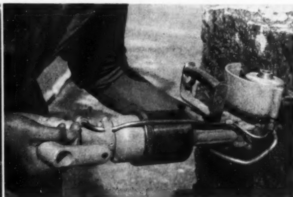
LEFT: The saw operated by a native is making a vertical test cut in a block of granite. The air hose is attached at the base of the handle; the water used as a coolant and to remove the cuttings flows through the tube alongside the air motor. RIGHT: Taking a horizontal cut. The supporting rod is not used, and one of the diamond saws has been removed.
